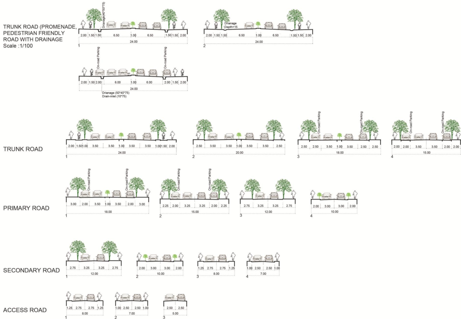
Figure 4.3 Cross-section examples for Urban Roads
